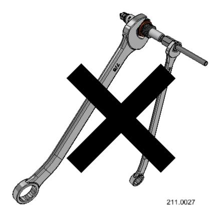
• DO NOT HOLD THE PROBE SHELL TO JAM THE JAM NUT.
