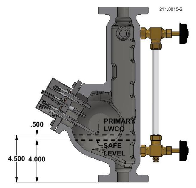
The Primary LWCO is 0.5 inches above the Minimum Safe Water Level specified by the boiler manufacturer.
