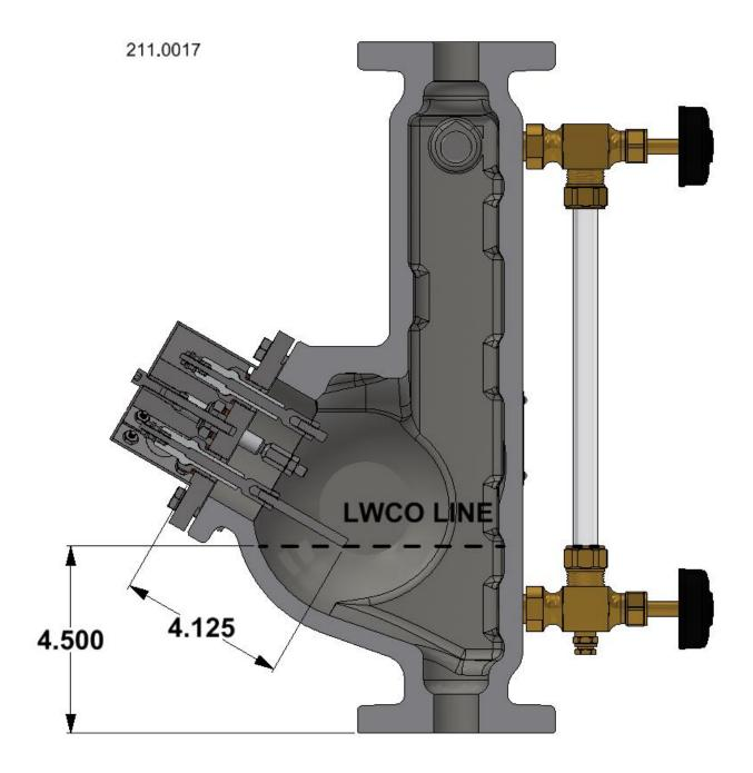
The LWCO ON level is factory set by the LWCO Probe (1). The LWCO Probe (1) is set at the top face of the bottom sight glass nut and should not be changed.
