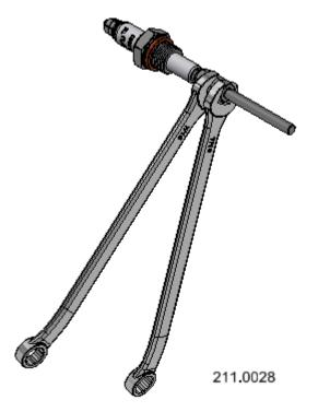
• Use 20ftlb torque to tighten the jam nut.
