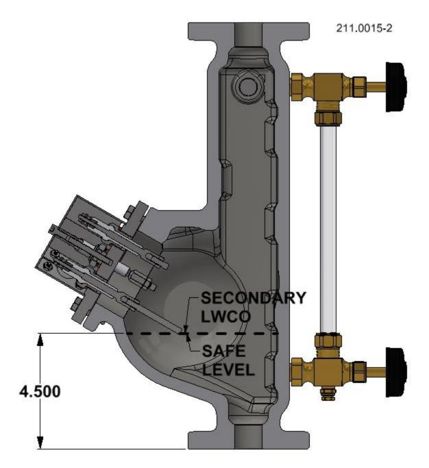
The Secondary LWCO ON Level must be installed at or above the Minimum Safe Water Level Specified by the Boiler Manufacturer. The Secondary LWCO ON Level is 4.5 inches above the LWCO bottom flange.
